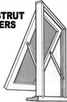
Gas strut hoppers operate the same as automobile hatchbacks and utilize gas strut mechanisms to hold the sash open. They can consequently enable quite wide openings in one controlled operation; ideal for bars or serveries.
