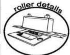
We use stainless steel spring loaded rollers mortised in the underside of each door to provide support & stability.
