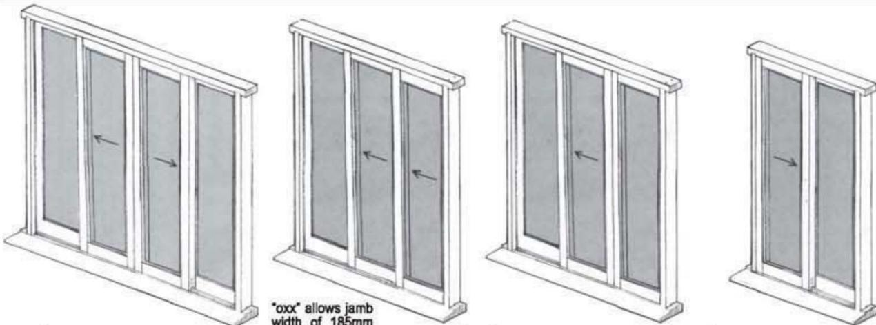
\*'xxx' allows jamb width of 185mm
