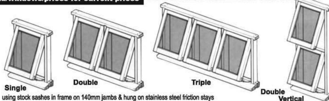
using stock sashes in frame on 140mm jambs & hung on stainless steel friction stays
