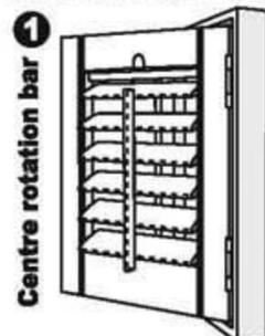
The bar is in the centre of the blade to the front of the shutter. This gives the best control and is best around kids.
