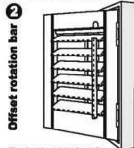
The bar is set to the left or the right of the blades, usually away from the centre of the opening. This works well on large openings to keep the centre clear.
